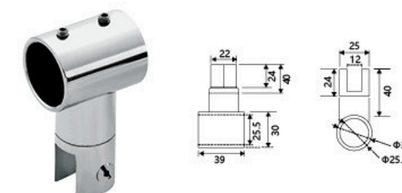
AT-E007 圓形穿管吊夾 Round pipe hanger
